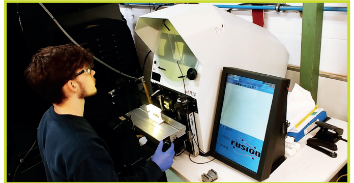
Quality checking a new batch of moulded components using the Baty Profile Projector
