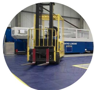
**Image 1: Trudec interlocking PVC tiles can be staggered to withstand constant movement of heavy roiling loads by forklift trucks and other industrial vehicles**
