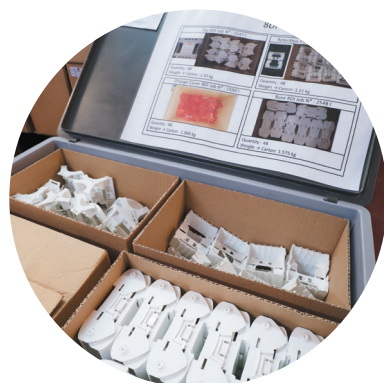
To boost productivity at Trend, Broanmain creates assembly kits, inserting components into reusable tubs.
