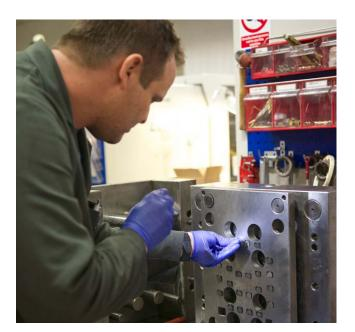
We now offer a standard maintenance/ service for our customers' tools. After an agreed timescale/cycle count, the tool is stripped, cleaned, polished and assessed for potential damage that may occur over the next period. This will provide our customers with a report on the status of the tool, and should enable us to predict where there might be problems during the next run.
