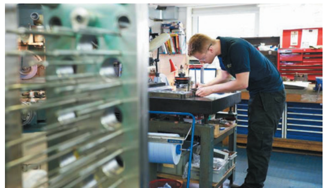
Making a tool in different parts rather than one solid piece means toolshop apprentice Kamil Stec can access any insert if changes need to be made
