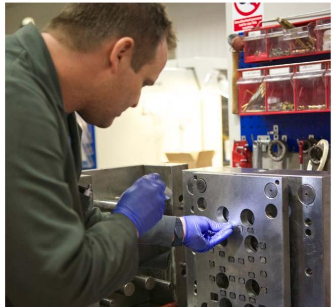
We now offer a standard maintenance/service for our customers' tools. After an agreed timescale/cycle count, the tool is stripped, cleaned, polished and assessed for potential damage that may occur over the next period. This will provide our customers with a report on the status of the tool, and should enable us to predict where there might be problems during the next run.
